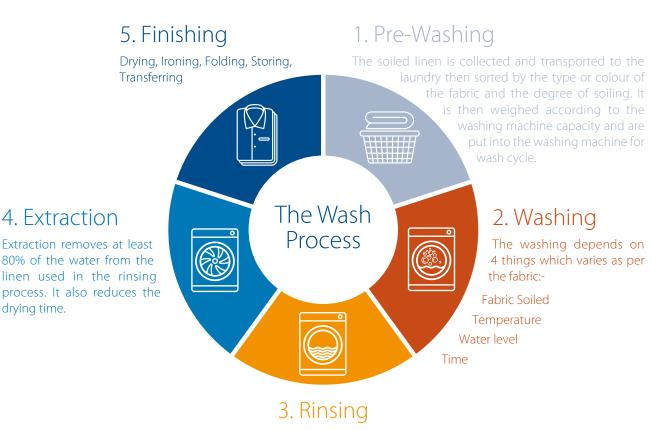
This is done by using hot and cold water, which are usually recovered & recycled from earlier steps during the last rinse in order to save water.
